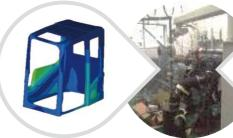
With vibration test bench and test bed, fuel tank and the cab has been tested by over hundreds of thousands of times on aspect of the vibration to improve the service life of the component by **50%**.
