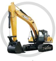
In allusion to the positions with concentrated stress such as oil vlinder connections and boom oot etc., special welding process and protection structure are used he stress on loading point is 20% wer than the competitor
