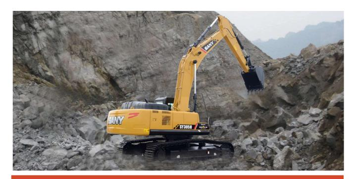
Worksite: Guizhou Working condition: Stonework (decomposed rock) Operating type: excavation- loading Work undertaken by SY305: Stone stripping, and loading
